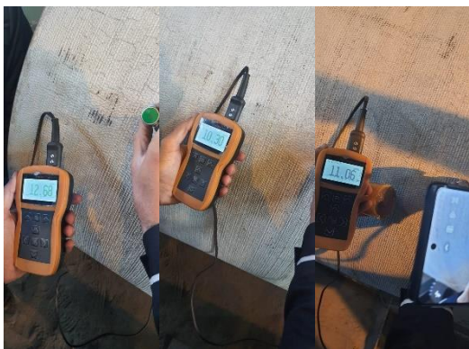
7.3 Dimension & appearance: dimensional requirement / wall thickness
