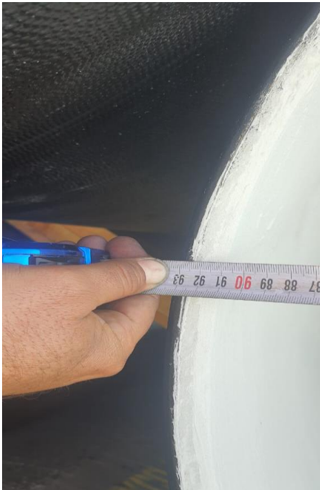
7.1 Dimension & appearance: External and Internal Socket
