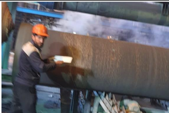
9. EXTERNAL COATING: Visual check
