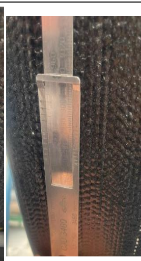
7.7 Dimension & appearance: internal diameter result
