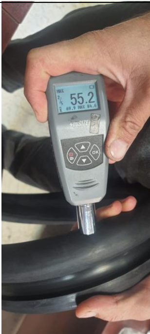
Soft section Hardness= 55 hard section= 84
