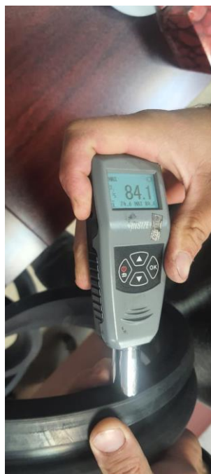
Soft section Hardness= 55 hard section= 84
