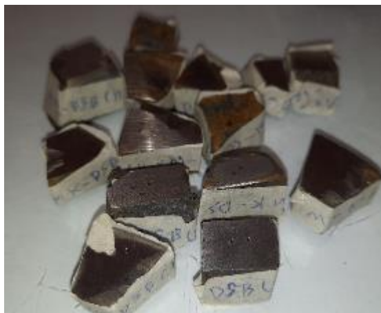
3. Fitting's microstructure & hardness sampling
