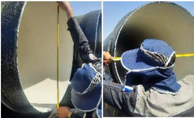
7.1 Dimension & appearance Control: External and Internal Socket Appearance
