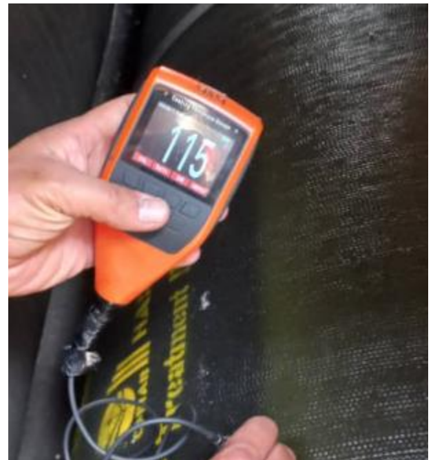
9.6 Coating thickness measurement
