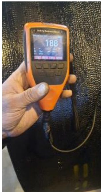
9.6 Coating thickness measurement
