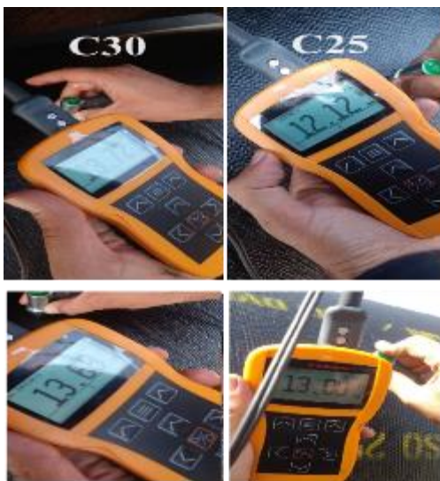
7.3 Dimension & appearance: dimensional requirement / wall thickness
