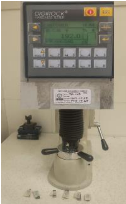
5. Mechanical properties-Brinell Hardness
